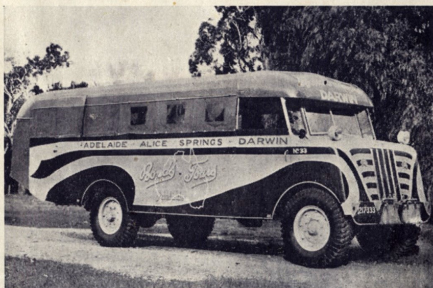
Bond's specially constructed four-wheel-drive coach, used for travelling over extremely rough and difficult terrain, is equipped with transmitting and receiving wireless units.
